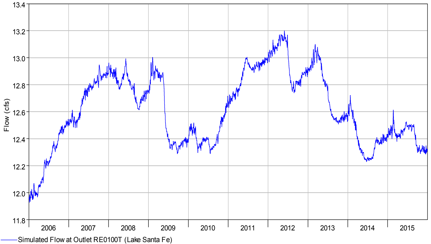
Figure 4-7B Simulated Groundwater Flow Hydrographs (2006-2015) - 2 of 3 Lake Alto and Lake Santa Fe Water Budget Modeling Suwannee River Water Management District
